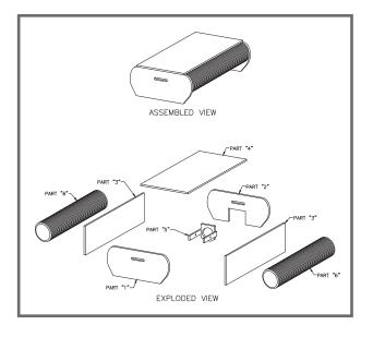
The Lane CQ is designed to be utilized in even the shallowest ponds. The smallest CQ, the 1.5" model requires only 3.5" of draft, meaning that it will function in only 3.5" of water above the bottom of the CQ float body.
