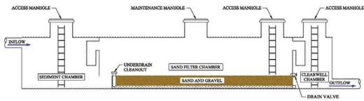
of a rain event. Periodically monitoring dewatering times will help determine when maintenance measures are needed. Standard maintenance operations include removing accumulated sediment and raking the first inch of sand. Usually, cultivating the top layer of sand will restore the drainage and filter characteristics of the filter bed, but at times the top few inches of media may require removal and replacement.
