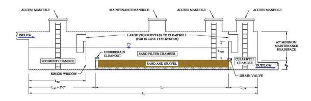
The controlling parameter associated with sand filter design is the water quality volume (WQv), obtained by multiplying a depth of rain water by the area tributary to the structure. The depth used varies among local storm water ordinances, and the tributary area often includes a reduction for pervious areas. The sediment chamber is typically sized to retain a percentage of the water quality volume (usually 25%) before spilling into the filter chamber.
